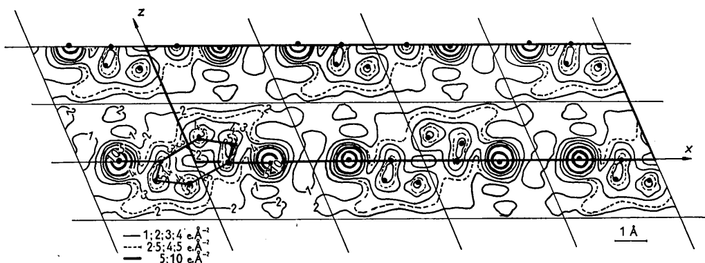
Fig. 2. Electron-density projection on absolute scale on the (010) plane calculated with the temperature factor with B = 4 \times 10^{-16} \text{cm}^2 . The schematic projection of a molecule is also represented. \bullet : peak of the function.
